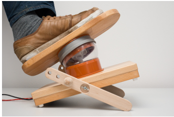
Figure 5: Foot-joystick : Two-axes foot-based tilting.
