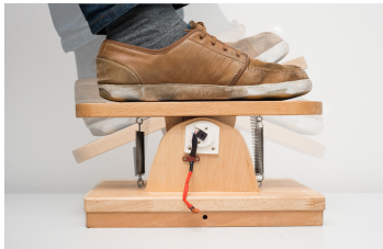
Figure 6: Foot-rocker : Two-directional foot pedal.
