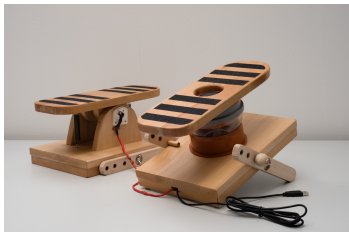
Figure 4: Foot-joystick & Foot-rocker setup
