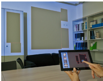
Figure 2: Demonstration tablet UI to drag and drop content into placeholders detected by our system (black frames on a blue background space).
