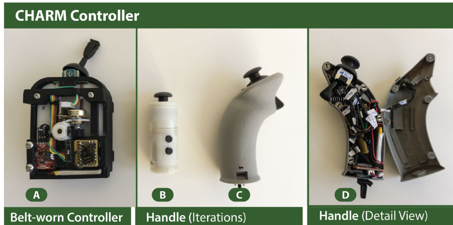
Fig. 3. Hardware prototype of our CHARM -Controller ( A ), showing the first ( B ) and second, ergonomic ( C ) iteration of our handle, as well as the hardware inside ( D ).
